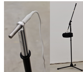
Figure 2: Picture of the App hardware setup: on the left: class 2-compliant external microphone, right: JBL Charge 5 Bluetooth loudspeaker.
